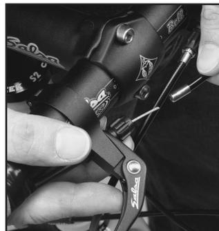
Reinsert the original brake cable through the drop-down handlebar lever, through the upper housing, and through the hole running through the center of the Cross Lever. Slide the cut off, lower part of the cable housing over the cable and insert the housing end (with housing ferrule attached) into the adjuster barrel of the Cross Lever. The other end of the housing runs to the brake. The effective housing length will increase slightly when adding the Cross Lever. Trim housing if you desire.
