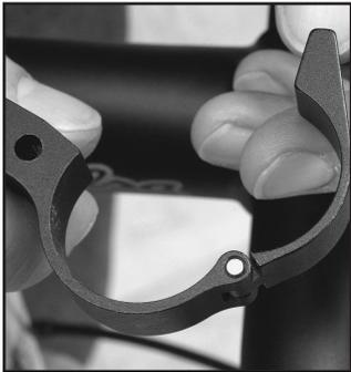
Salsa Cross Levers are designed to be mounted onto 31.8mm diameter (or 26.0mm diameter via included shim) drop-down handlebars. The hinged clamp design of Salsa Cross Levers allows the lever to be mounted and installed without having to remove handlebar tape or the original brake levers.
