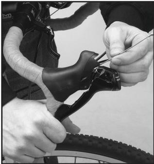
Detach the brake cable from the brake as per manufacturer's direction. Remove the brake cable from the cable housing as per the original lever/brake manufacturer's instructions. The housing may remain in its original position inside the handlebar grip tape.
