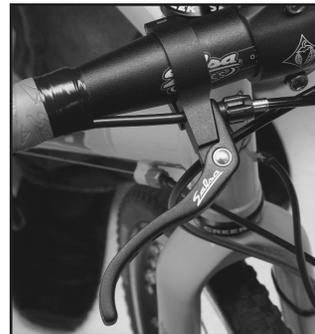
Attach the housing & cable to the brake, and set up the brake according to the manufacturer's instructions.
