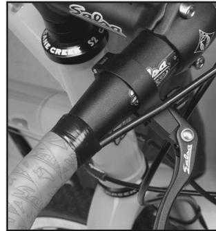
Open the hinged clamp of the Cross Lever by unscrewing the clamping bolt with a 4mm Allen wrench. Place the Cross Lever on the 31.8 (or 26mm handlebar via shim) handlebar. Close the hinge clamp and insert the clamping bolt. Before tightening, position and angle the lever to a comfortable and convenient position on the bars. Tighten the clamping bolt with a 4mm Allen wrench. Final tightening torque is 6-8Nm.
