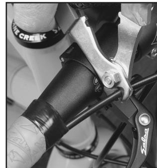
Cut the cable housing at a position where it reaches the top mount lever clamp on the side that is furthest away from the center of the handlebar (see photo). Insert the upper housing end into the housing guide hole on the clamp.
